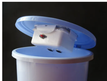
Figure 6 Detection sensor installation
